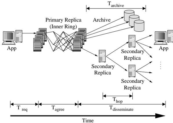
Figure 2: *The path of an OceanStore update.* An update proceeds from the client to the primary replica for its target data object. There, it is serialized with other updates and applied to that target. A heartbeat is generated, certifying the new latest version, and multicast along with the update down the dissemination tree to other replicas. Simultaneously, the new version is erasure-coded and sent to archival storage servers.
