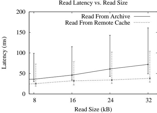
Figure 6: *Latency to Read Objects from the Archive.* The latency to read data from the archive depends on the latency to retrieve enough fragments for reconstruction.
