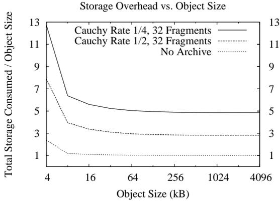
Figure 4: *Storage Overhead*. Objects of size less than the block size of 8 kB still require one block of storage. For sufficiently large objects, the metadata is negligible. The cost added by the archive is a function of the encoding rate. For example, a rate 1/4 code increases the storage cost by a factor of 4.8.
