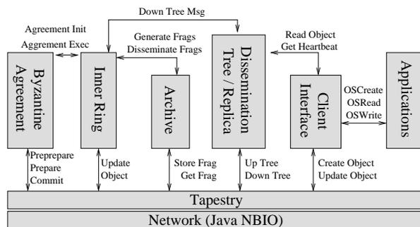
Figure 3: *Prototype Software Architecture*. Pond is built atop SEDA. Components within a single host are implemented as *stages* (shown as boxes) which communicate through events (shown as arrows). Not all stages run on every host; only inner ring hosts run the Byzantine agreement stage, for example.
