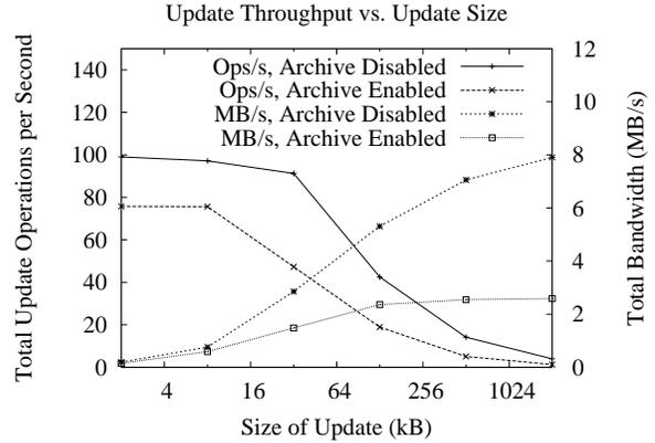
Figure 5: *Throughput in the Local Area.* This graph shows the update throughput in terms of both operations per second (left axis) and bytes per second (right axis) as a function of update size. While the ops/s number falls off quickly with update size, throughput in bytes per second continues to increase. All experiments are run with 1024-bit keys. The data shown is the average of three trials, and the standard deviation for all points is less than 3% of the mean.
